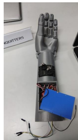
A Model of the Smart hand developed by PSG iTech students
