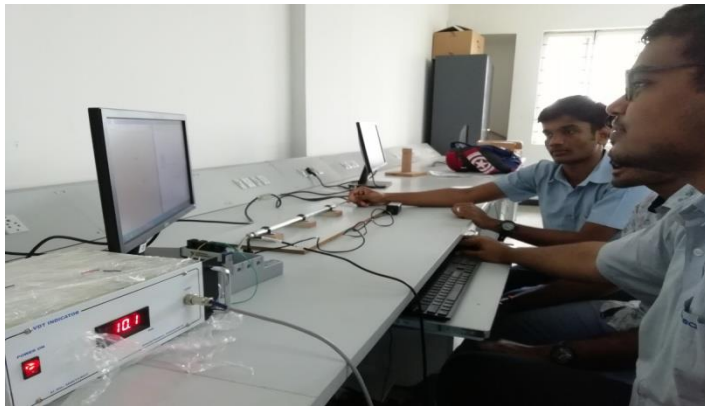
Students were interfacing the LVDT with Computer using DAQ
